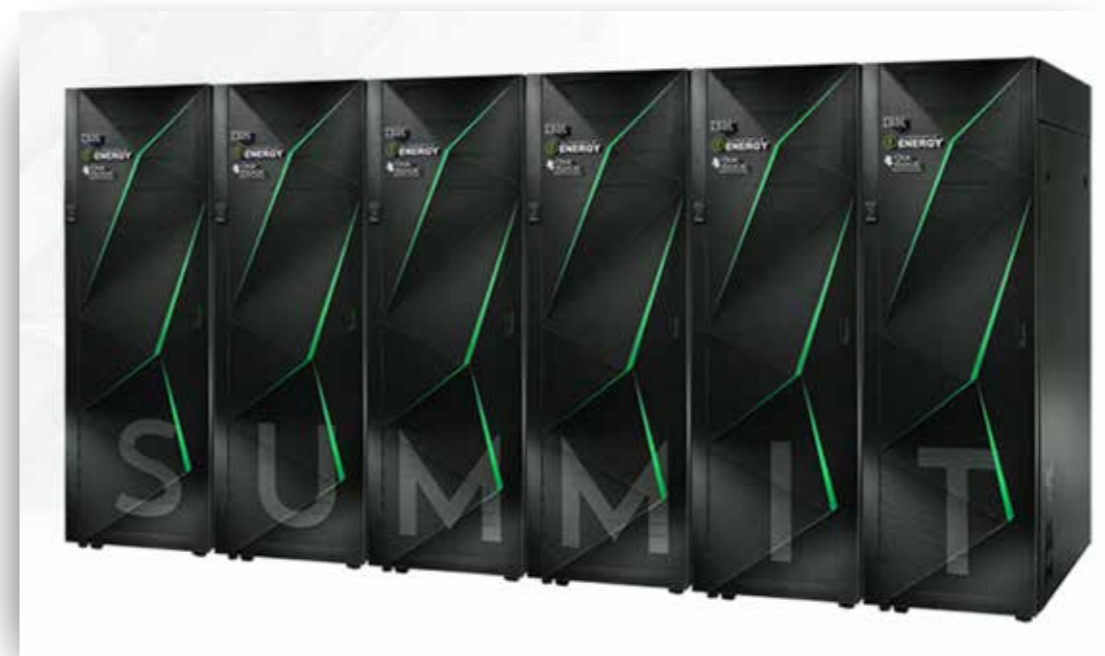
ORNL's next-generation supercomputer SUMMIT, x5 faster, 4086 nodes The goal is ~9 s, ultimately 1 s ( exascale era ).
