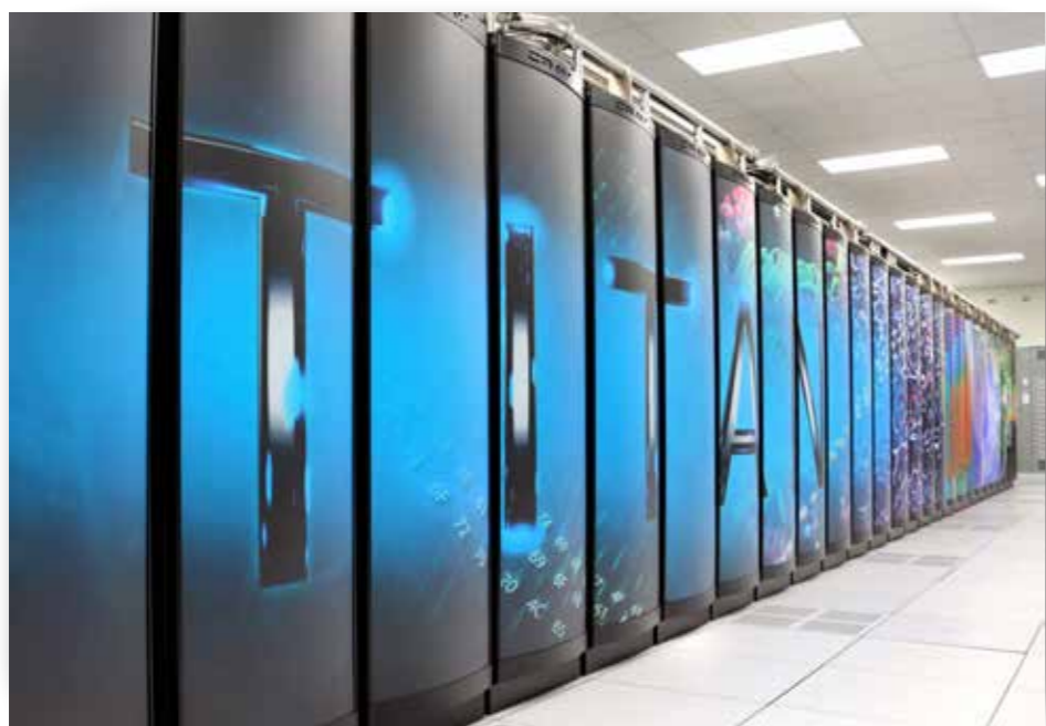
ORNL's Cray XK7 TITAN system 16,384 GPUs
