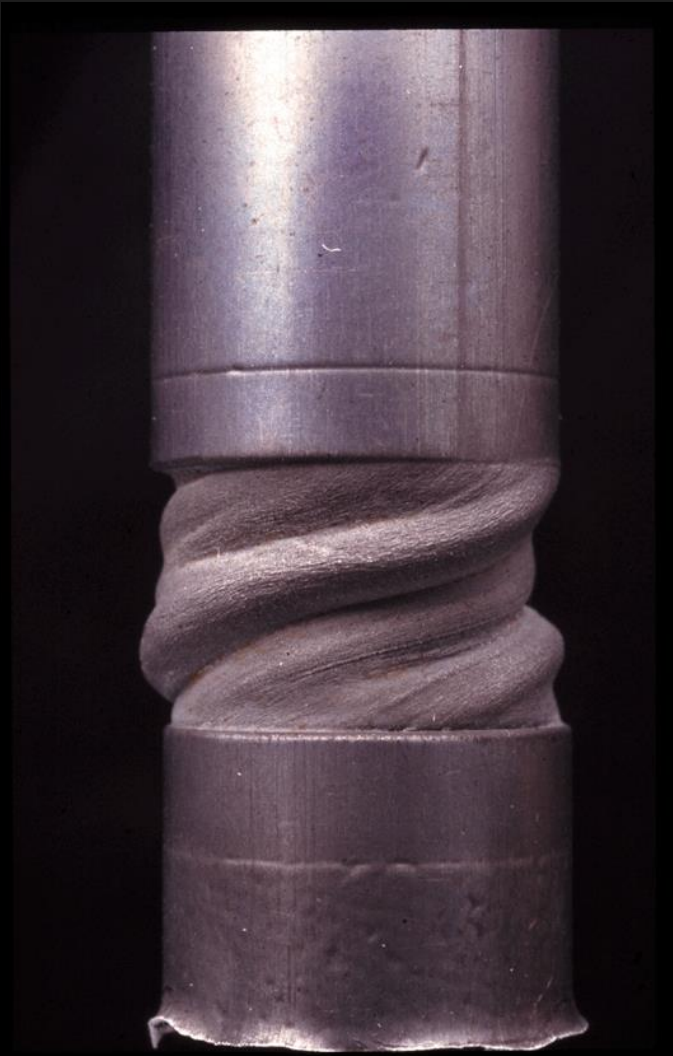
Marble deformed in torsion (L. Burlini)
